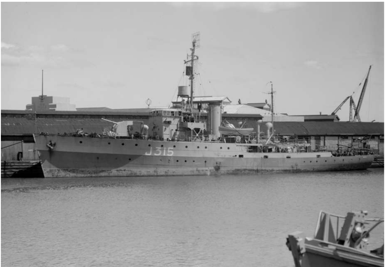
HMAS Wagga in Melbourne following her return to Australia in 1945. Note that she is riding high in the water, having been defueled, as preparations are made to place her in Reserve status.
